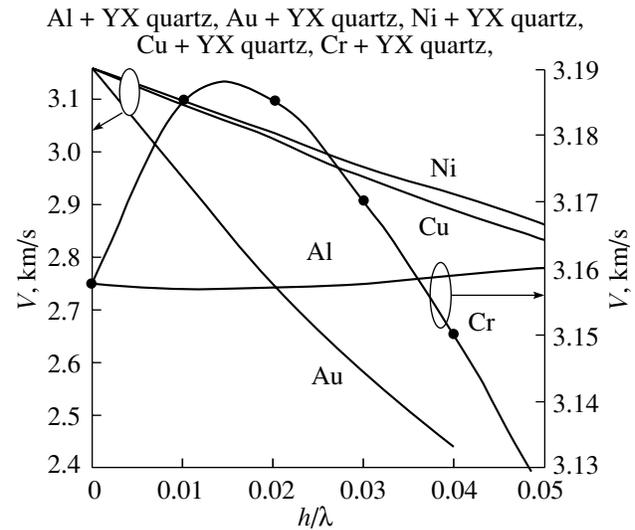
**Fig. 3.** Dependences of the SAW velocity on the relative layer thickness in the structures: Al film + YX-cut SiO<sub>2</sub>; Au film + YX-cut SiO<sub>2</sub>; Ni film + YX-cut SiO<sub>2</sub>; Cu film + YX-cut SiO<sub>2</sub>; and Cr film + YX-cut SiO<sub>2</sub>.
