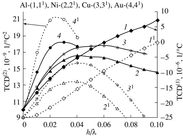
**Fig. 1.** Dependences of the coefficients  $TCD_1^{(1)}$  (solid curves) and  $TCD_1^{(2)}$  (dotted curves) of SAW on the relative layer thickness for different metal films on the surface of a YX-cut quartz crystal: (1, 1<sup>1</sup>) Al, (2, 2<sup>1</sup>) Ni, (3, 3<sup>1</sup>) Cu, and (4, 4<sup>1</sup>) Au.
