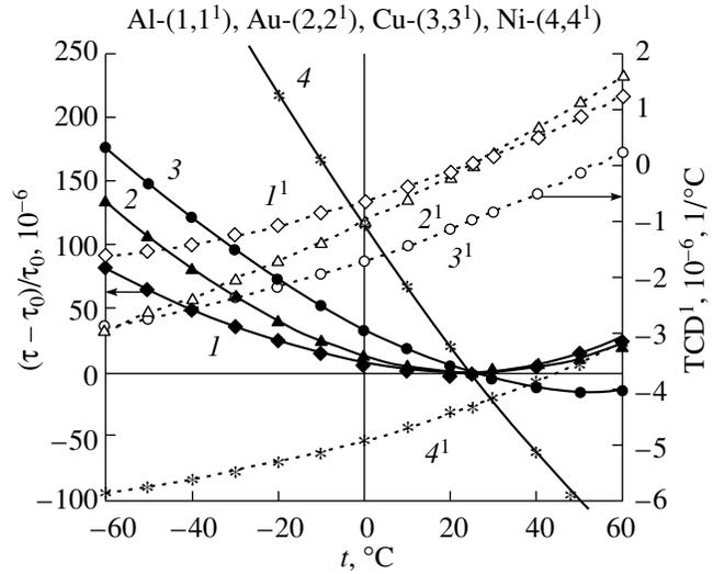
**Fig. 2.** Temperature dependences of the relative variation of the delay time  $\Delta\tau/\tau_0$  (solid curves) and the coefficient  $TCD_1^{(1)}$  (dotted curves) of SAW for different films deposited on the surface of a YX-cut quartz crystal: (1, 1<sup>1</sup>) Al film with  $h/\lambda = 0.061$ , (2, 2<sup>1</sup>) Au with  $h/\lambda = 0.028$ , (3, 3<sup>1</sup>) Cu with  $h/\lambda = 0.05$ , and (4, 4<sup>1</sup>) Ni with  $h/\lambda = 0.045$ .
