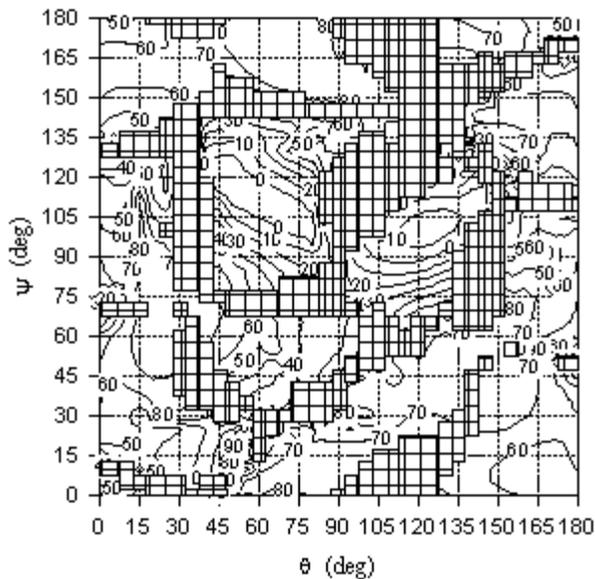
Figure 5: Temperature coefficient of delay (ppm/°C) for  $\phi = 20^\circ$ .
