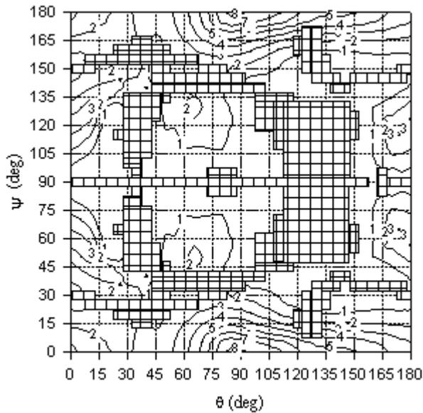
Figure 2: Coupling coefficient (%) for  $\phi = 0^\circ$ .
