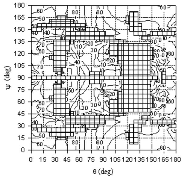
Figure 3: Temperature coefficient of delay (ppm/ $^\circ\text{C}$ ) on open surface for  $\phi = 0^\circ$ .
