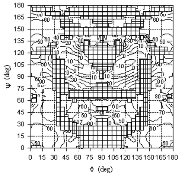
Figure 6: Temperature coefficient of delay (ppm/°C) for  $\phi = 30^\circ$ .
