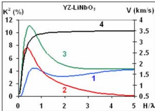
Fig. 1a. Dependences of  $K^2$  (curves 1, 2, 3) and velocity (curve 4) on normalized plate thickness. Zero symmetric mode.
