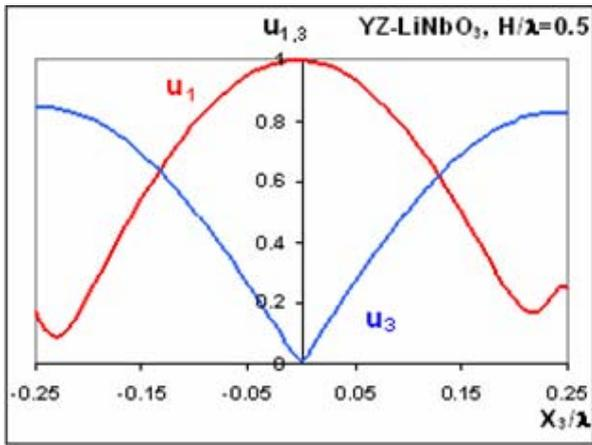
Fig. 2. Distribution of mechanical displacements along the plate thickness.
