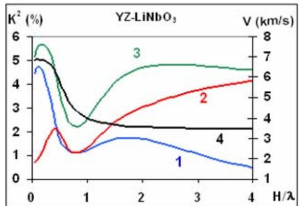
Fig. 1b. Dependences of  $K^2$  (curves 1, 2, 3) and velocity (curve 4) on normalized plate thickness. Zero anti-symmetric mode.
