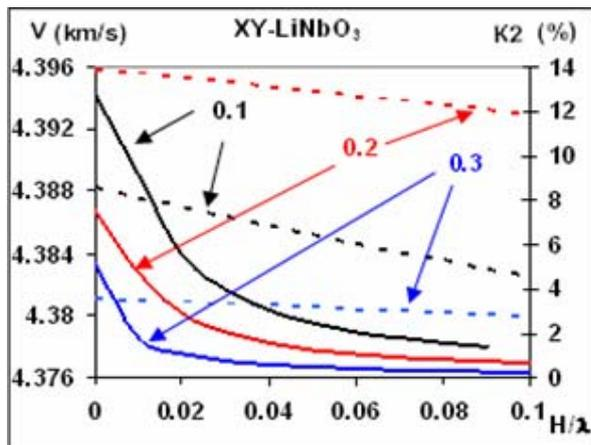
Fig. 4. Dependences of velocity (dotted lines) and  $K^2$  (solid lines) on normalized gap width.
