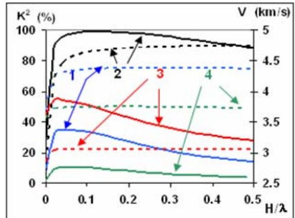
Fig. 3. Dependences of velocity (dotted lines) and  $K^2$  (solid lines) on normalized plate thickness.
