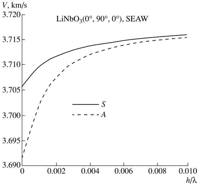
**Fig. 2.** Dependence of the phase velocity  $V$  on  $H/\lambda$  for the (A) antisymmetric and (S) symmetric modes of the SEAW in a system of two identical piezoelectric media, YX-cut LiNbO<sub>3</sub>.
