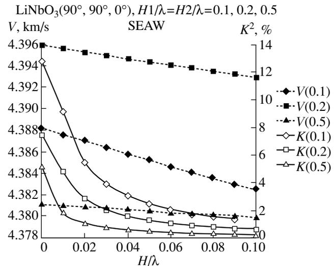
**Fig. 9.** Velocity  $V$  of the fast mode of the SEAW (curves  $V(0.1)$ ,  $V(0.2)$ , and  $V(0.5)$ ) and the electromechanical coupling coefficient  $K^2$  (curves  $K(0.1)$ ,  $K(0.2)$ , and  $K(0.5)$ ) as functions of the gap width  $H/\lambda$  for three values of the piezoelectric plate thickness:  $H1/\lambda = 0.1, 0.2$ , and  $0.5$ .
