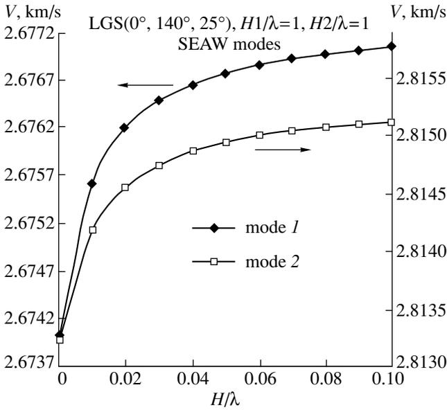
**Fig. 7.** Dependences of the velocities of the symmetric and antisymmetric modes of SEAW (modes 1 and 2) on  $H/\lambda$  in a system of two piezoelectric plates made of langasite (LGS) with the orientation (0°, 140°, 25°).
