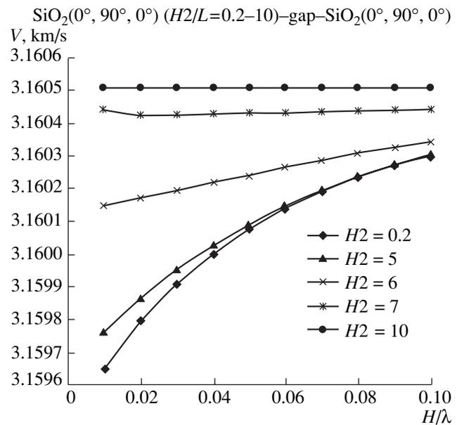
Fig. 4. Dependence of the phase velocity of the SEAW on  $H/\lambda$  in a system consisting of a YX-cut SiO<sub>2</sub> piezoelectric plate and a YX-cut SiO<sub>2</sub> piezoelectric medium with a gap between them for different values of the plate thickness:  $H_2 = 0.2, 5, 6, 7,$  and  $10$ .
