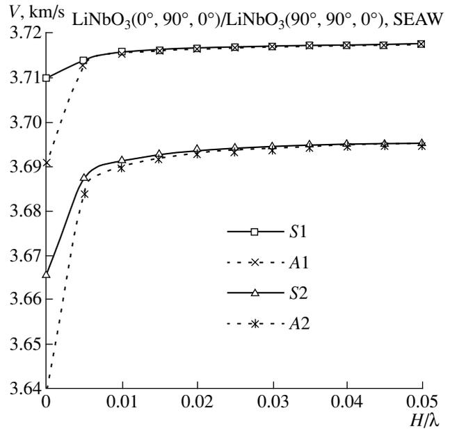
**Fig. 3.** Dependence of the phase velocity of the SEAW modes on  $H/\lambda$  in a system of two piezoelectric media: YX-cut LiNbO<sub>3</sub> and XY-cut LiNbO<sub>3</sub> with a gap between them.
