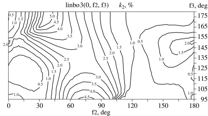
**Fig. 3.** Lines of equal value for  $K^2$  in the  $\text{LiNbO}_3$  crystal ( $f_1 = 0^\circ$ ,  $f_2 = 0^\circ\text{--}180^\circ$ , and  $f_3 = 95^\circ\text{--}180^\circ$ ).
