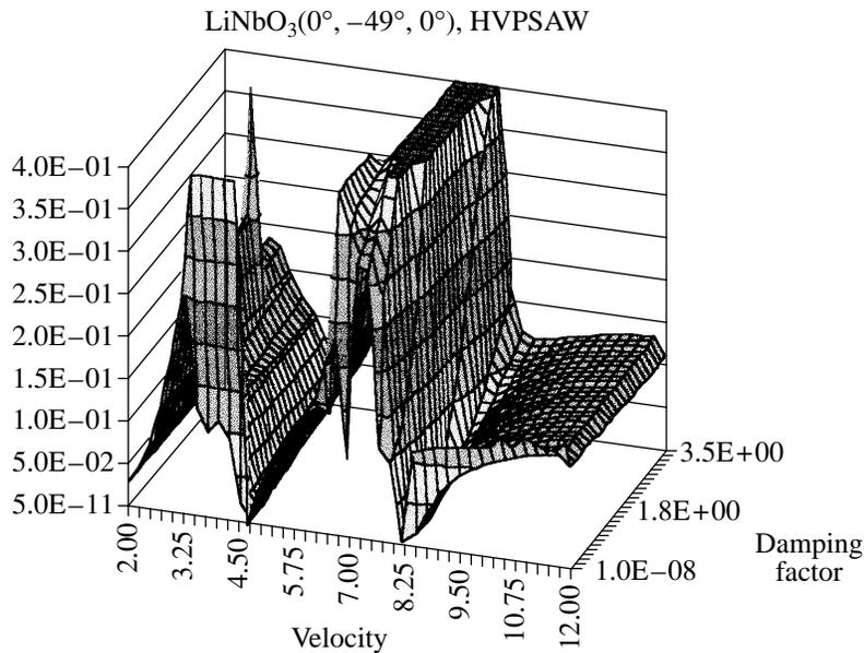
**Fig. 2.** Relief of the target function  $F(V, \delta)$  used in the search for an HVPSAW solution in a LiNbO<sub>3</sub> crystal with the (0°, -49°, 0°) orientation.
